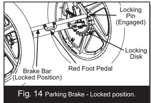
Fig. 14 Parking Brake - Locked position.
