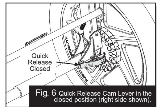
Fig. 6 Quick Release Cam Lever in the closed position (right side shown).
