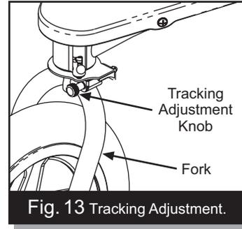
Fig. 13 Tracking Adjustment.
