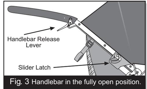
Fig. 3 Handlebar in the fully open position.
