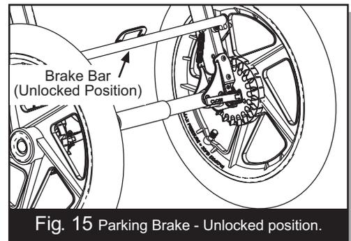
Fig. 15 Parking Brake - Unlocked position.
