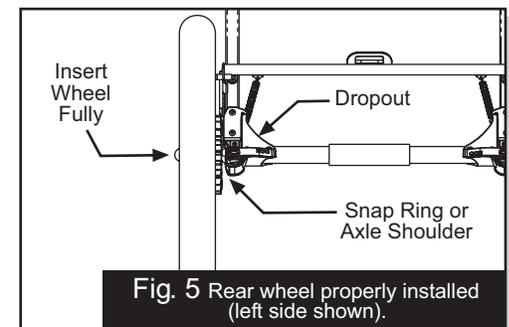
Fig. 5 Rear wheel properly installed (left side shown).
