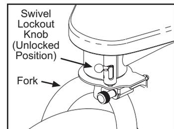
Fig. 10 Swivel Lockout - Unlocked Position (Walk Mode)
